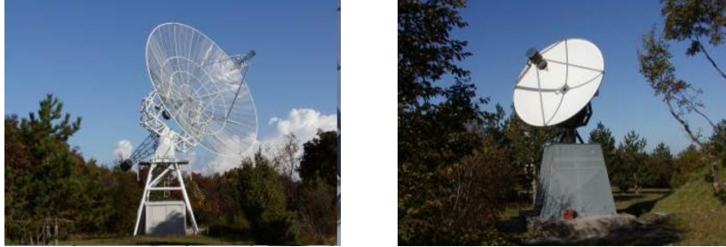
Figure 2.1: The TSRS 1.0 system. It was a set of two multi-channel radio polarimeters, which were detecting the solar radio emissions in the metric band by a 10-meter diameter parabolic dish (left panel), and in the decimetric one by a 3-meter parabolic dish (right panel), at the following frequencies 237, 327, 408, 610, 1420, 2695 MHz, with very high temporal resolution (1 ms standard) and accurate circular polarisation measurements. It is not longer operational due to a lightning stroke that irreparably compromised its operations in 2010.
