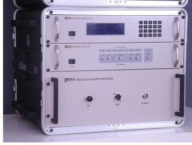
Figure 2.5: POAM Electronics ACU and ADU controllers (first two elements on the top) and SDR receiver (last element on the bottom).
