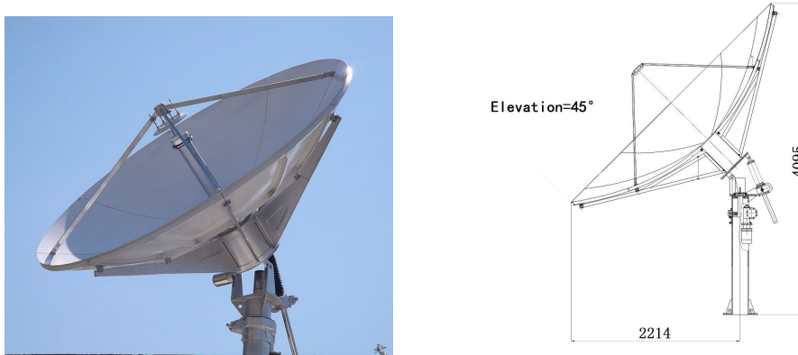
Figure 2.3: The left panel shows 3-m antenna by POAM. The right panel depicts the mechanical structure.
